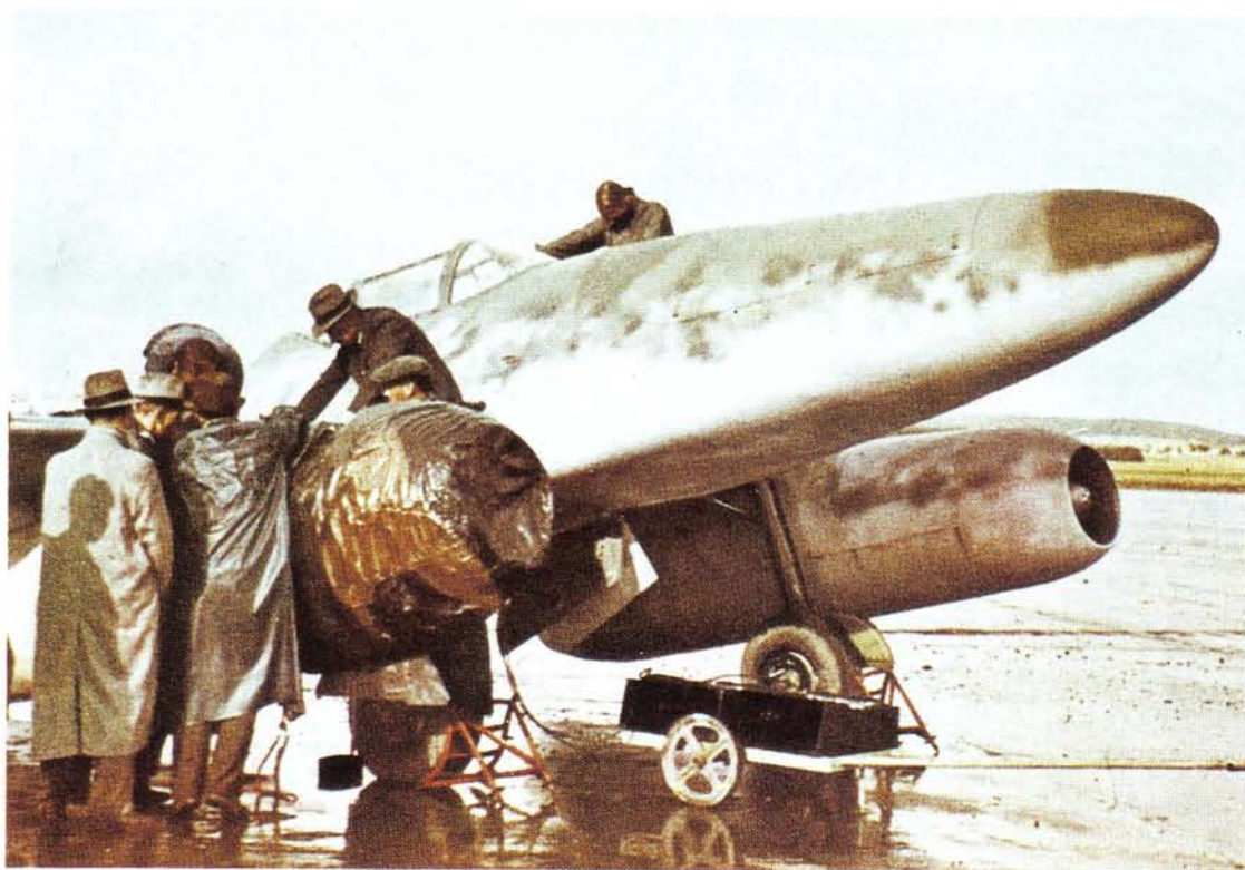
The Me 262 V3 was powered by Jumo 004 turbojets and was equipped with a tailwheel undercarriage.
