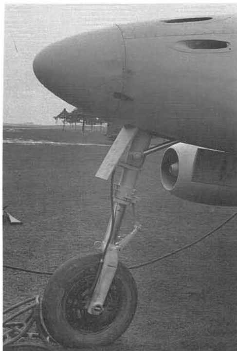
The Me 262 V6 (VI+AA, WNr. 130 001), the first Me 262 with an hydraulically-retractable nose-wheel and Jumo 004 B engines. Drawing by Th. Mohr.
