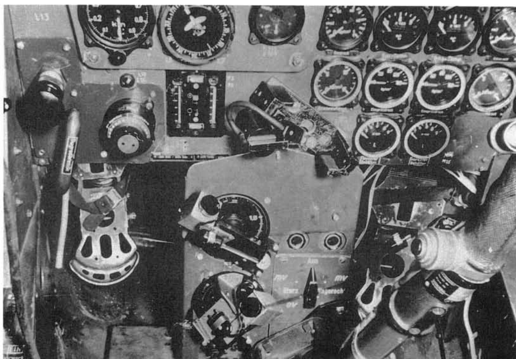
Installation of the semi-programmable Low-level and Dive-bombing System (TSA) in the Me 262 A-1a/U1 fighter-bomber.
