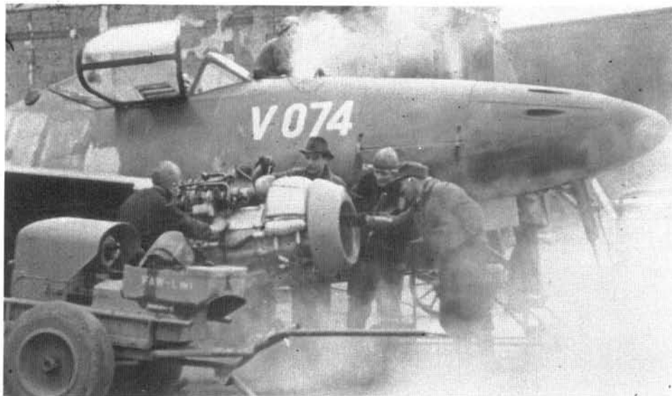
The Me 262 V074, prototype for the C-1b version (the "B" indicated the use of BMW engines) or Heimatschützer (Interceptor II). The aircraft, which was powered by two BMW 003 A-1 jet engines with superimposed BMW 109-718 liquid fuel rocket motors, was photographed during a successful static engine run on March 23, 1945.
