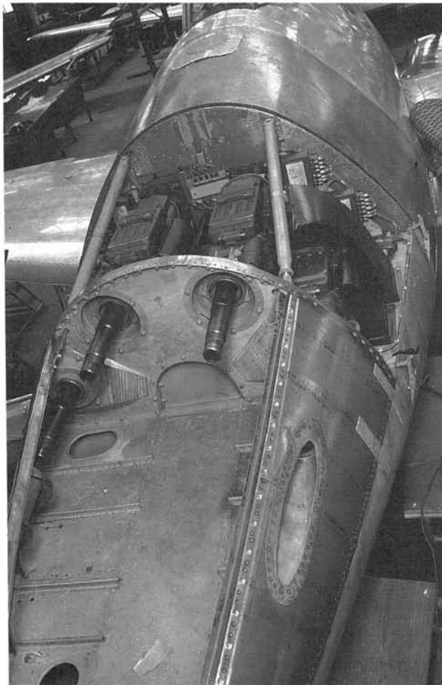
Fuselage nose with weapons installation before and after attachment to the fuselage.
